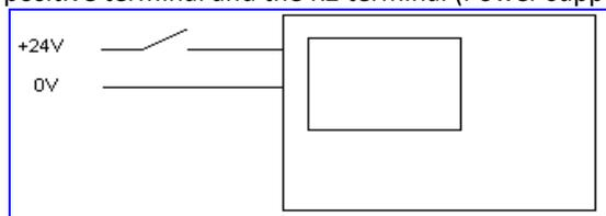
*Note: If the K3 (0V) terminal is disconnected and the bus bar voltage is applied to the MASTER 2.0, there is the risk of getting AC voltage on the CANBUS terminals.*
