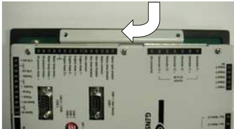
Figure 21 - Mounting brackets on MASTER 2.0
