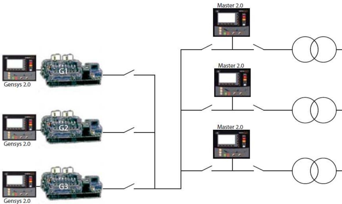
**Figure 17 - Paralleling with several mains**
