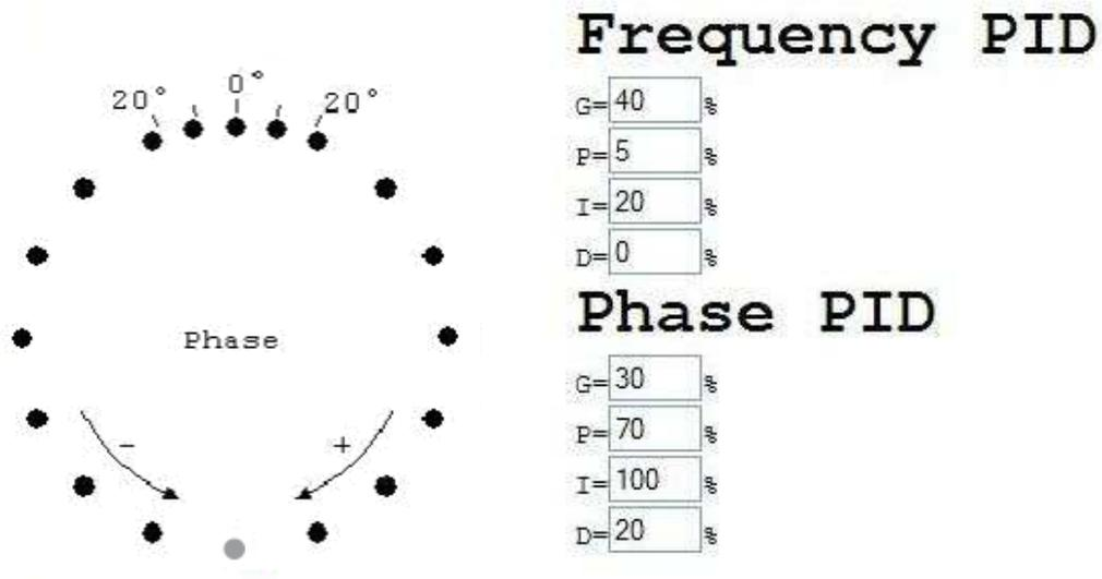
Figure 47 – Synchroscope frequency & phase PID
