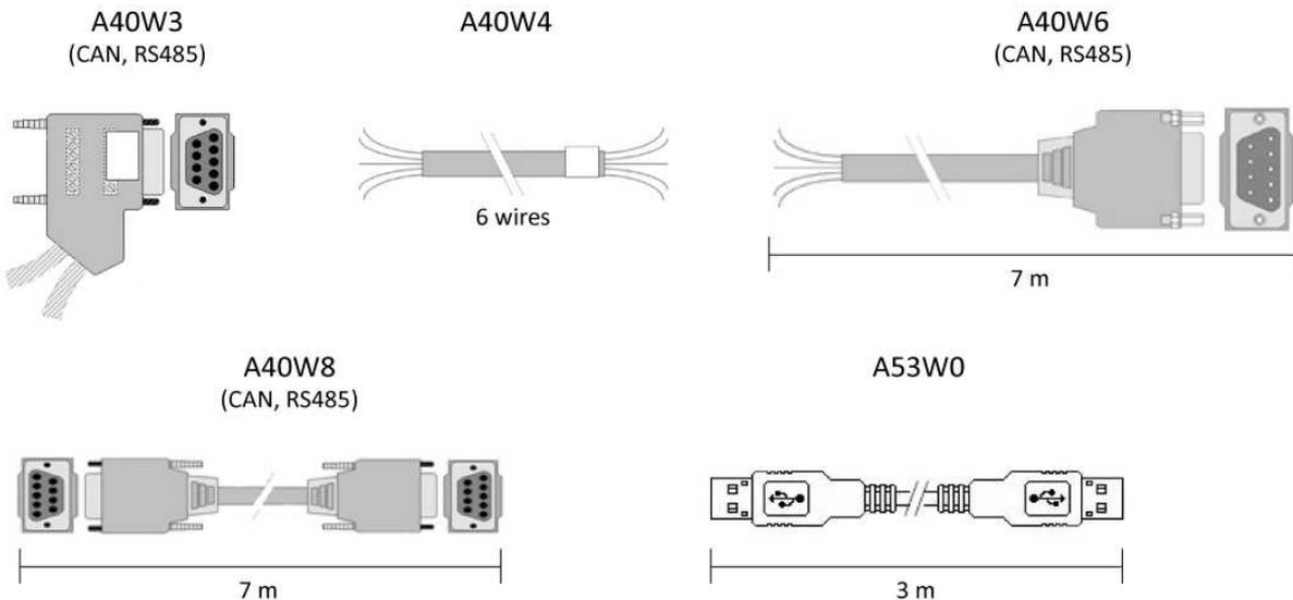
Figure 58 - Standard cables
