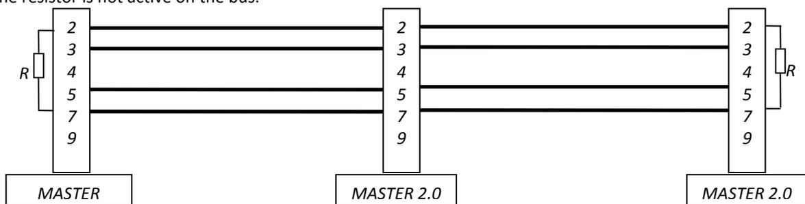
Figure 31 - CAN Bus wiring
