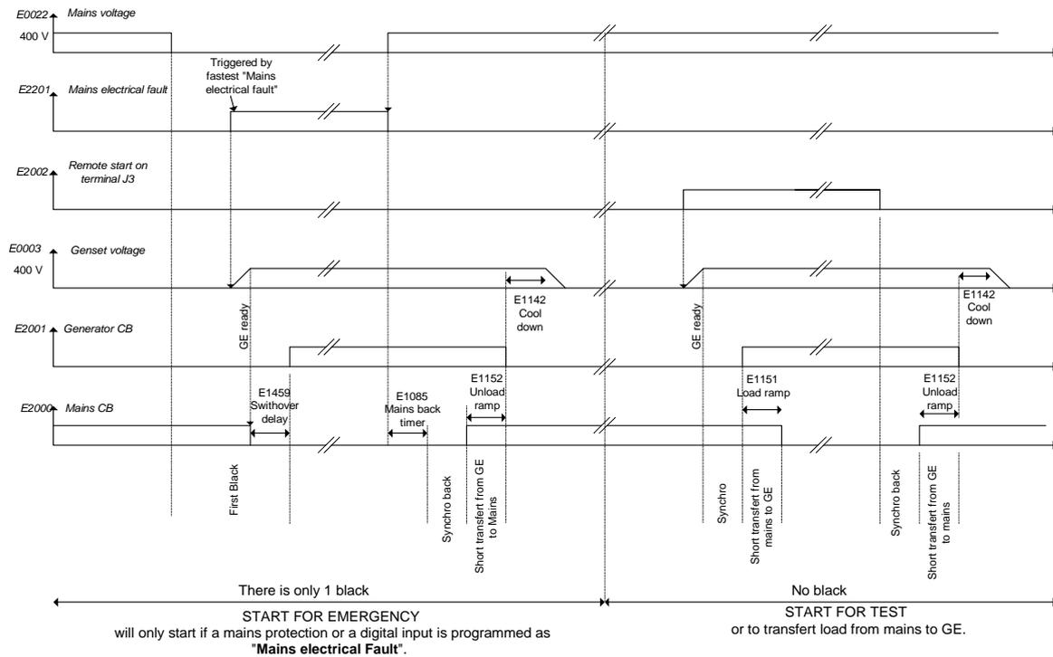
**Figure 15 - Typical sequence in No Break CO mode**
