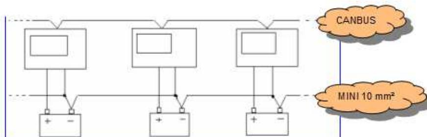
**Figure 23 - Interconnection of all battery negatives**
