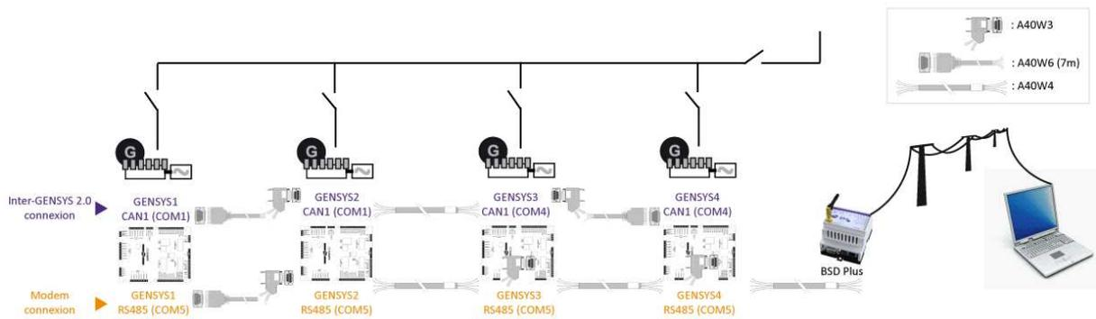
**Figure 37 - MASTER 2.0 ↔ MASTER 2.0 ↔ MASTER 2.0 ↔ ... (MODBUS)**
