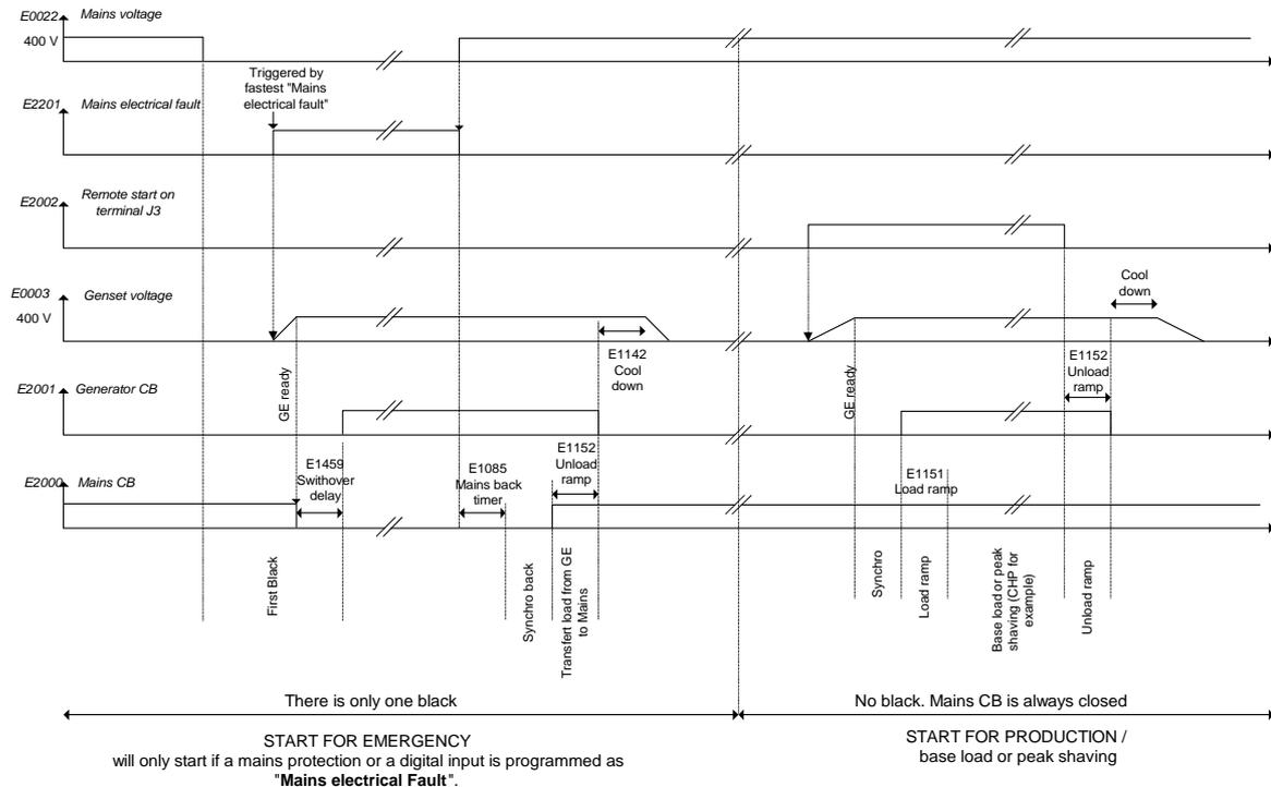
Figure 16 - Typical sequence in permanent mode
