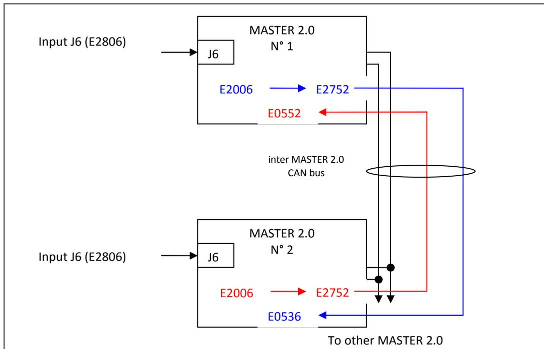
**Figure 34 - Connecting J6 to broadcast variables**
