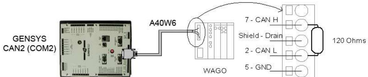
**Figure 36 - CANopen coupler wiring**
