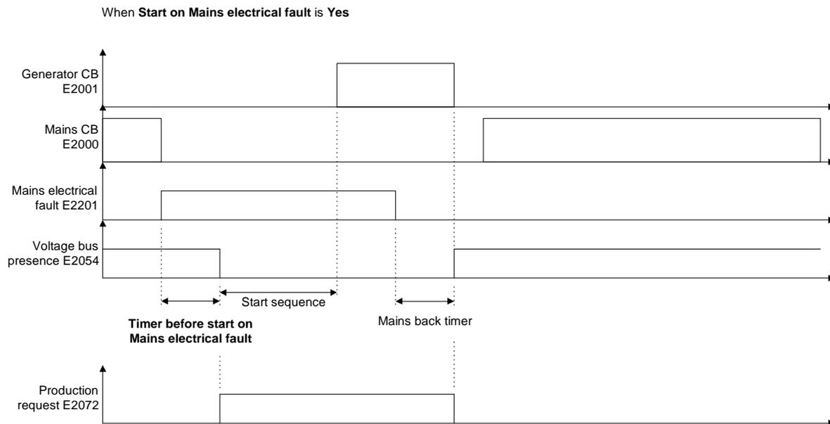
**Figure 24 - Change over with one digital input programmed as "Mains electrical fault"**
