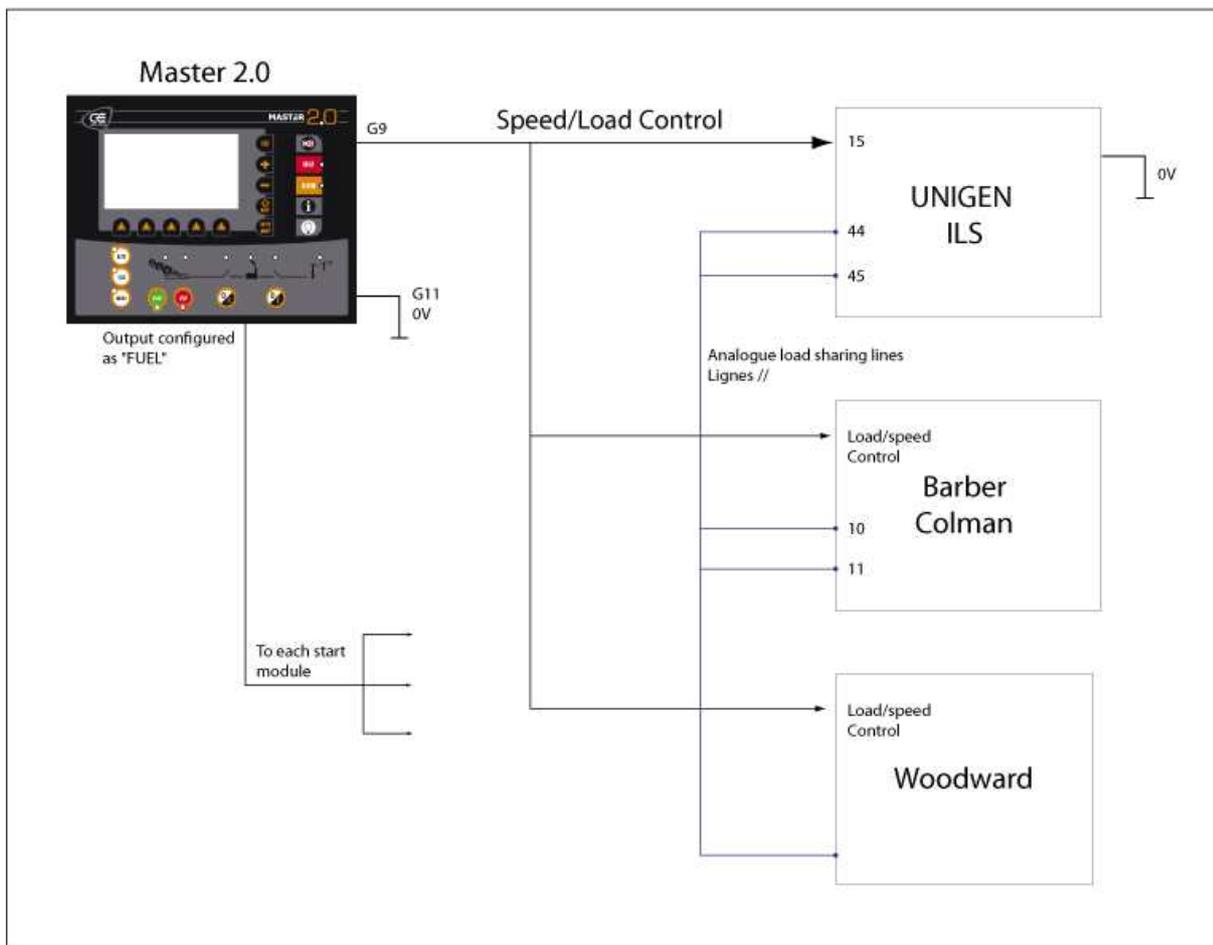
Figure 18 – Load sharing with MASTER 2.0 and parallel line modules
