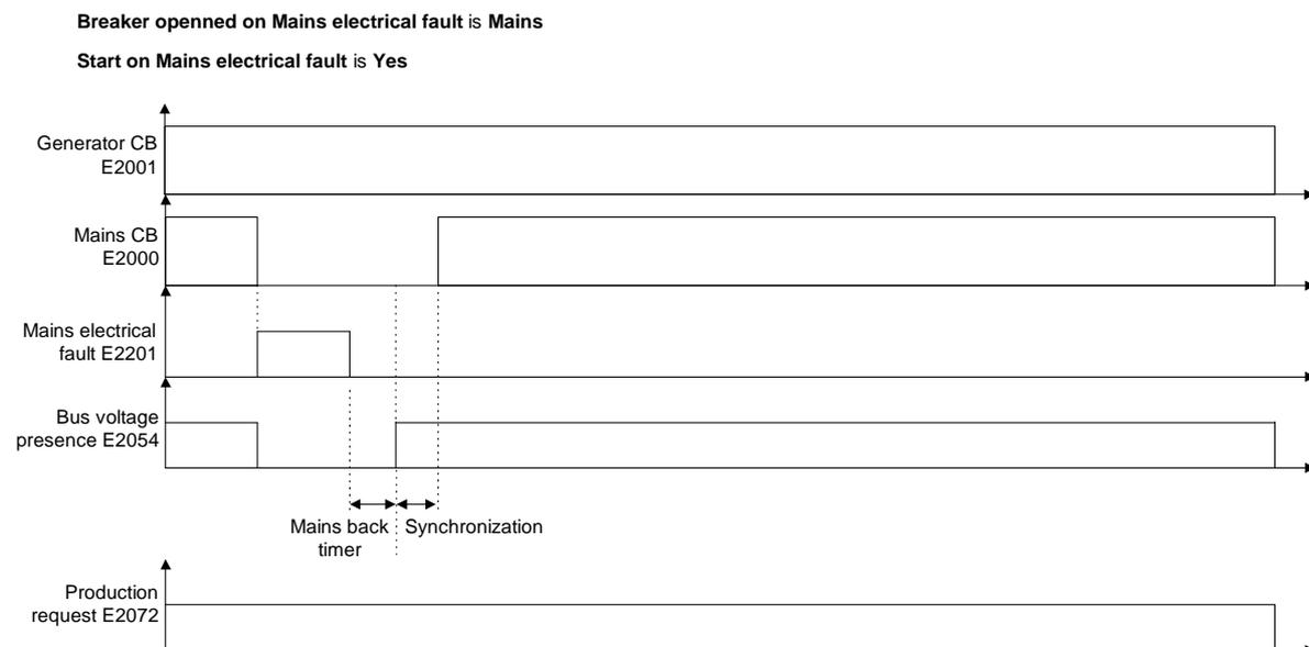
**Figure 25 - Permanent mains paralleling with one digital input programmed as "Mains electrical fault"**
