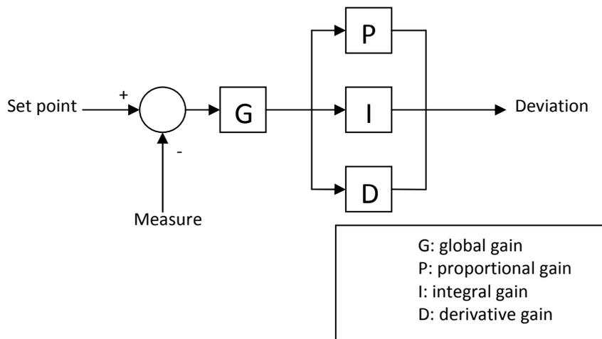
**Figure 29 - Typical GPID controller**
