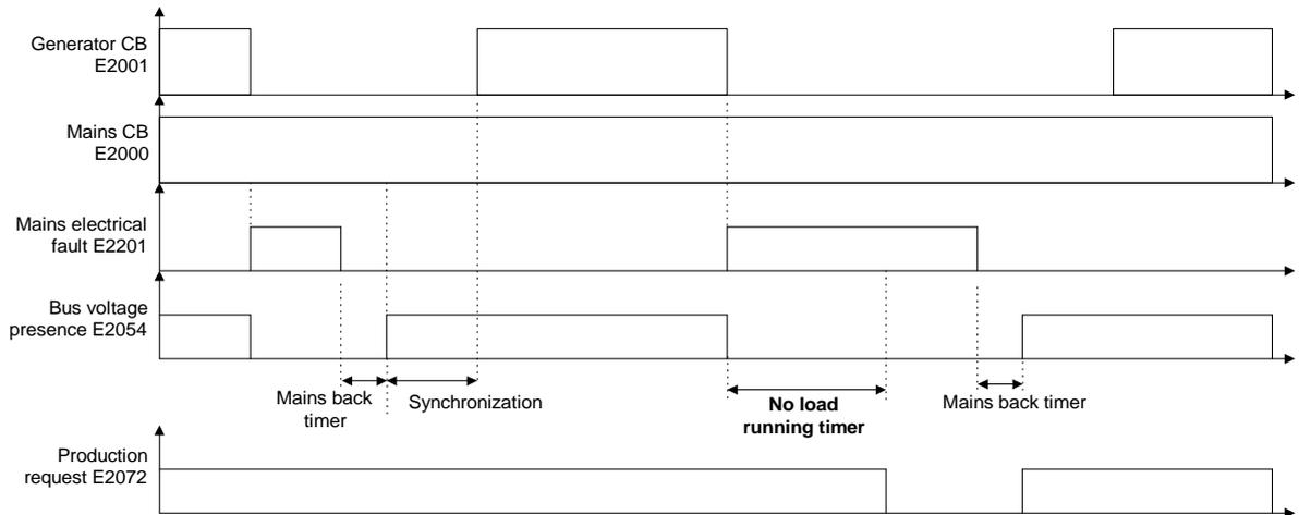
Figure 26 - Permanent mains paralleling with one digital input programmed as "Mains electrical fault"
