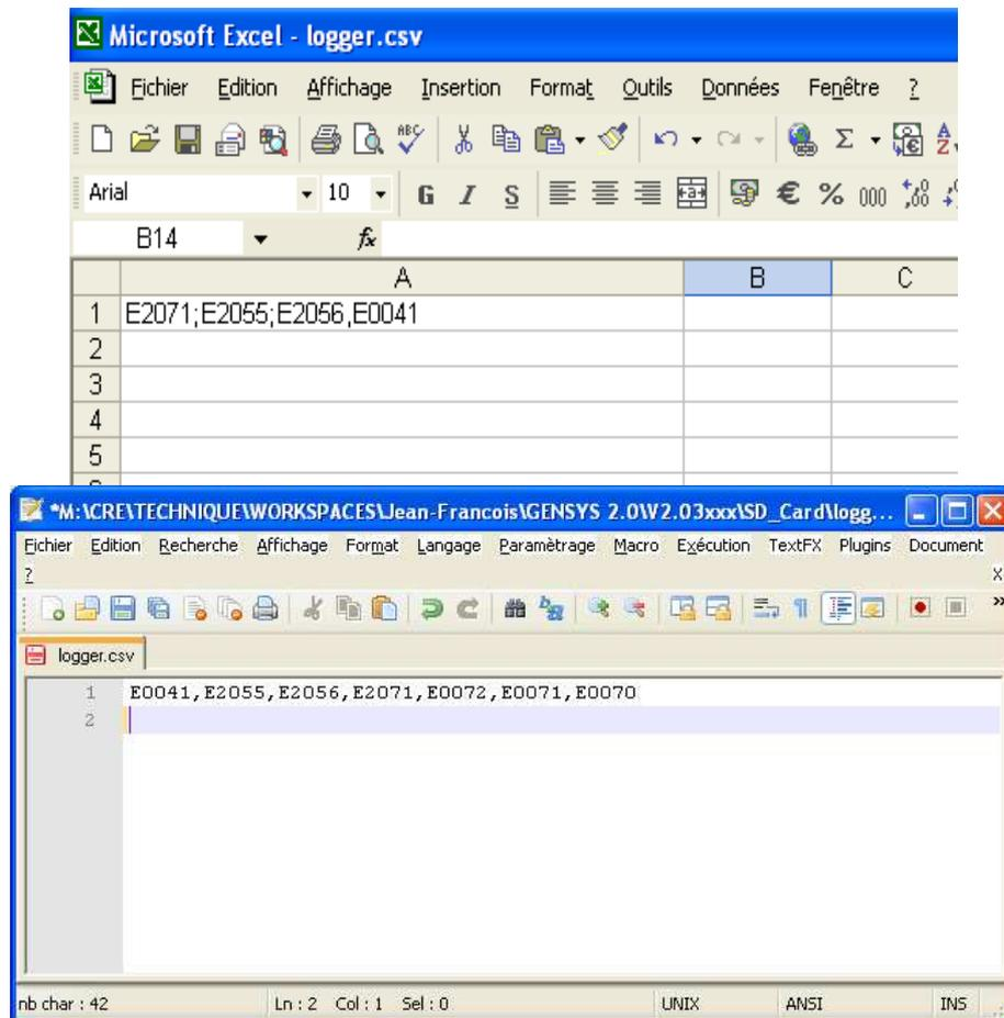
Variable E4041 allows you to choose the recording time in seconds. As soon as the SD card is inserted into the MASTER 2.0, the recording will start every E4041 seconds.
