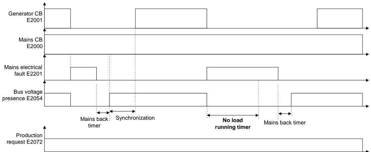
Figure 27 - Permanent mains paralleling with one input as "Mains electrical fault"
