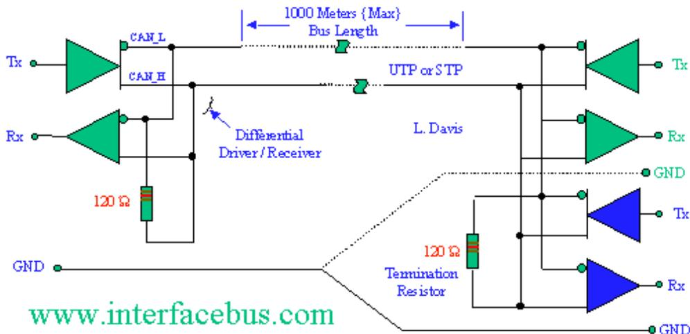
Figure 30 – CAN bus wiring
