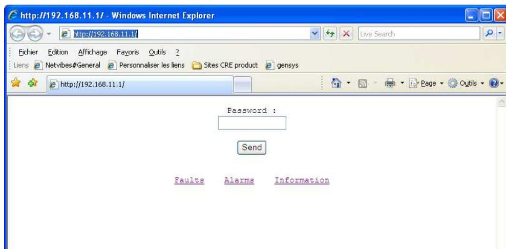
Note: Parameter E4042 allows the user to set the connexion time in minutes. Once this time is passed, the password will be asked for again.
