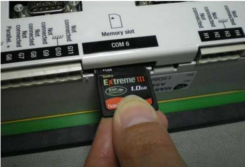
Memory cards must be FAT16 format and no larger than 2Go. High capacity SDHC cards and FAT32 format are not compatible.
